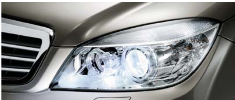
The Intelligent Light System includes bi-xenon headlamps and active cornering light function
